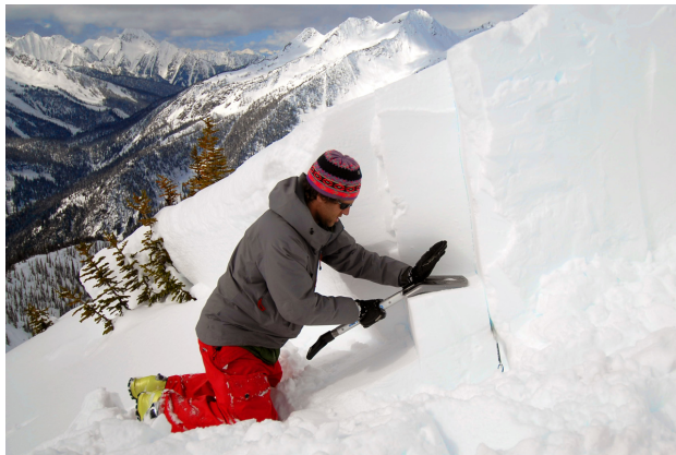
Figure 1. Deep Tap Test (DT). A block of 30 cm by 30 cm by 15 cm above the persistent weak layer is isolated. The test is completed by applying 10 taps moving the hand from the wrist, 10 taps moving the arm from the elbow, and 10 taps moving the arm from the shoulder. The number of taps and the fracture character are recorded.
