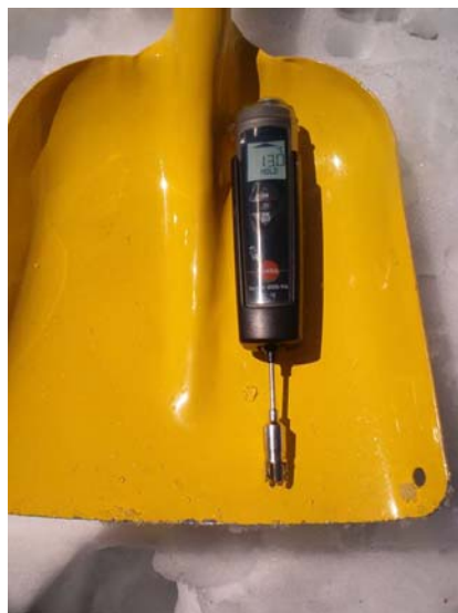
Figure 3.5: Testo 825-T4 infrared thermometer used to make manual measurements of snow surface temperature at each array site (photo: ASARC).
