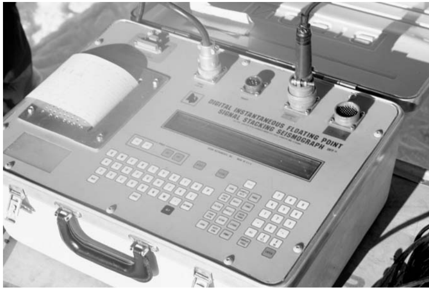
Figure 3.8 Bison geophone recorder used to measure velocity of fracture propagation in a weak snowpack layer. ASARC photo.
