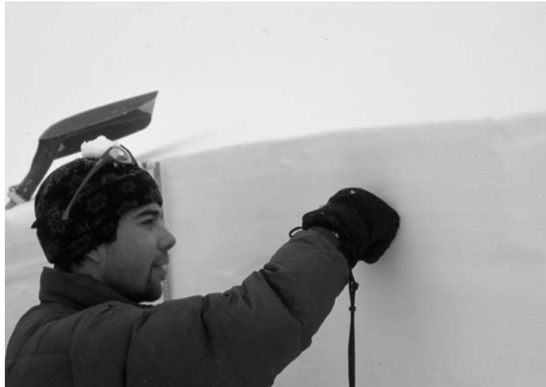
Figure 1.7 Inserting a fist into the snowpack to determine the layer's hand hardness . ASARC photo.
