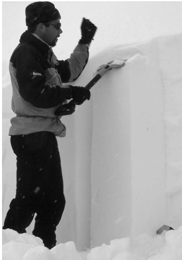
Figure 3.5 Compression test technique. ASARC photo.
