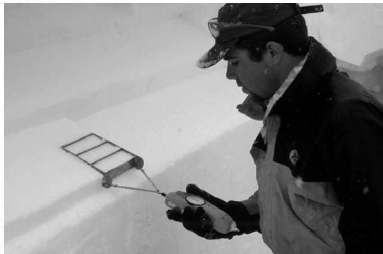
Figure 3.4 Shear frame technique. ASARC photo.
